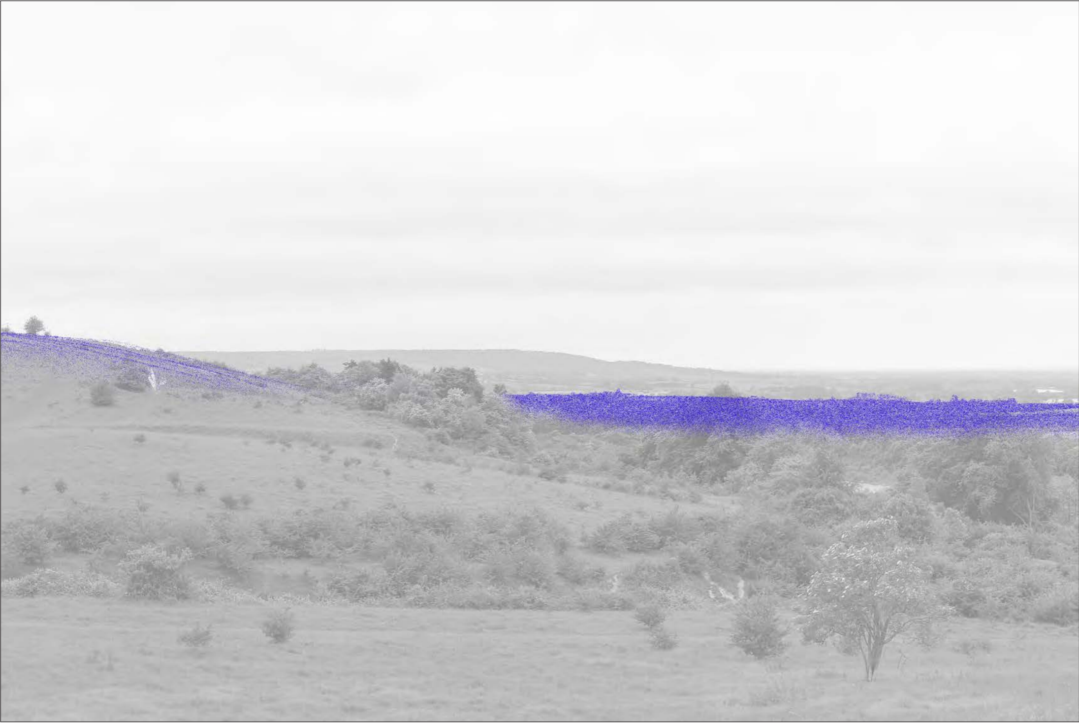
Survey Reference Points - LIDAR Point Cloud Alignment on existing photography
